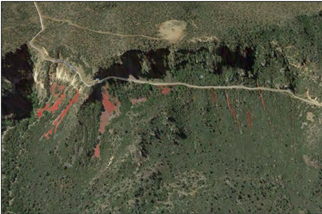
**Figure 3-14. Red highlights indicate areas of recent rockfall, rock avalanche, and debris flow activity**
